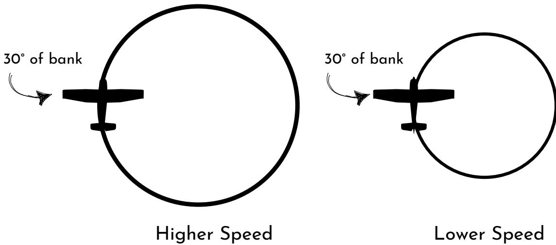
**Rate of Turn** - A turn flown at a higher airspeed will have a slower rate of turn than a turn flown at a slower airspeed. Therefore, to complete a standard rate turn of 360° in 2 minutes (3° per second), the higher the airspeed, the steeper the required bank angle.
